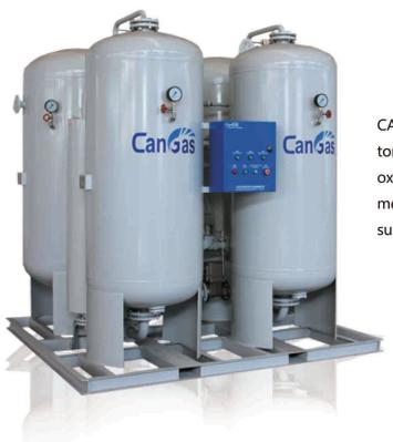
CANGAS® CAPO-HP 99+% oxygen generator applies PSA technology to make oxygen with Maximum purity up to 99+%. It meets requirements for the applications such as steel cutting and so on.
