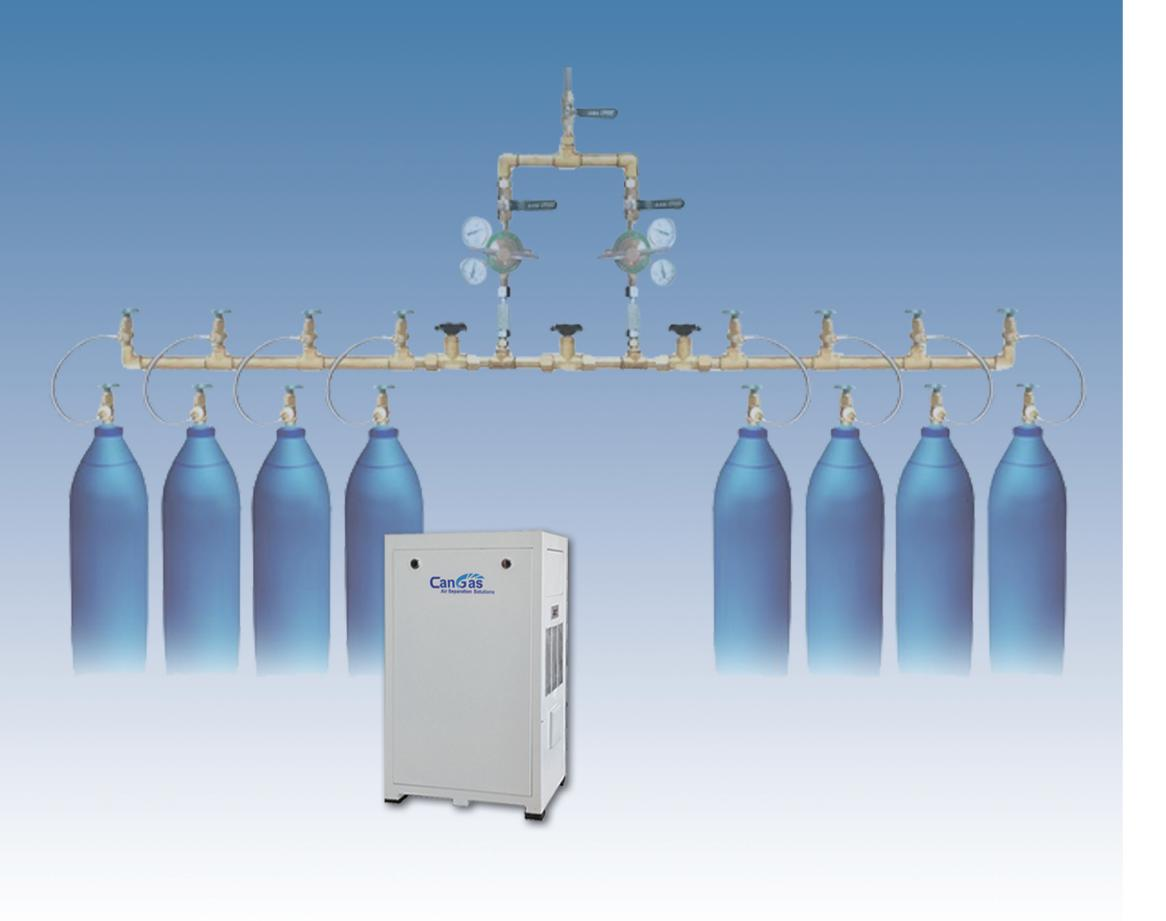
MICROCFS C series  $O_2$  system has been developed specially for the requirement of safe, reliable and convenient  $O_2$  generation and  $O_2$  compression. The MICROCFS C series incorporates PSA  $O_2$  generation unit,  $O_2$  compression and cylinder filling unit with design features for a variety of industrial and medical applications, is suitable for the compression of  $O_2$  up to 150bar, The MICROCFS will fill up to 4 cylinders (40Liter) in a 24 hours period.
